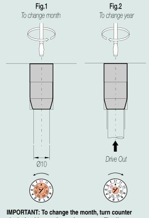
clockwise (the two inner rings move, Fig. 1). To change the year, turn clockwise (only central ring moves, Fig. 2). Catalog Number
