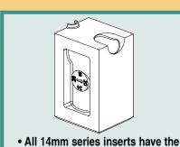
All 14mm series inserts have the full 360 degree 'a' dimension molded into one side of the insert for easy reference
