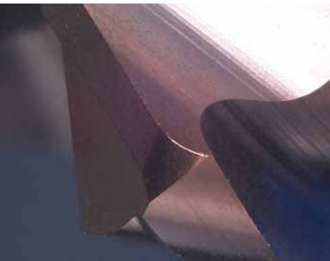
Strong and thick gash corner
