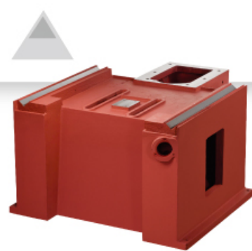
Precision ground and Turcite "B" coated. Extra wide double "V" ways on the cross slide to increase machine rigidity and grinding accuracy.
