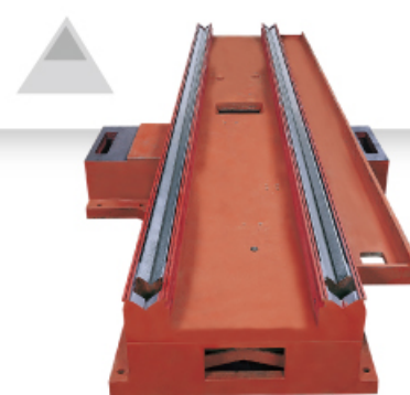
Column type base utilizes double "V" slideways on the table that are hand scraped and Turcite "B" coated for greater rigidity and smoother movement.
