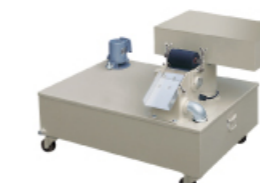
Cooling System with Magnetic Separator
