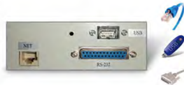
▪ The USB Port allows to upload and download through Flash drive.
