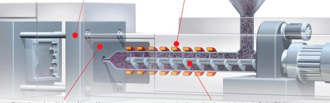
Resin exits nozzle and is injected into mold. During a purge the nozzle is pulled back and resin is pushed out. Once the new resin comes out without any specks or streaking, the molding machine is put back into service. Heater bands cover barrel to melt plastic resin. Resin will bake onto the barrel and bits of old resin will flake off, which will impact quality. Over time resin "bakes on" barrel and screw.
